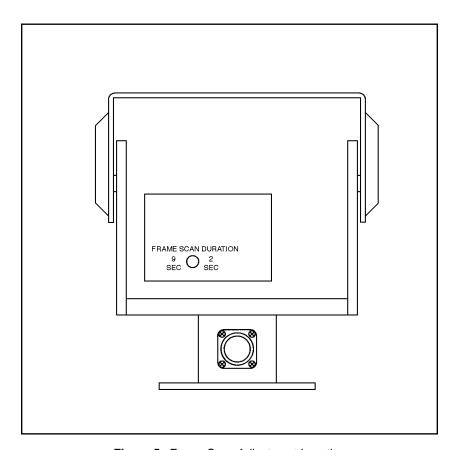
Figure 5. Frame Scan Adjustment Location
